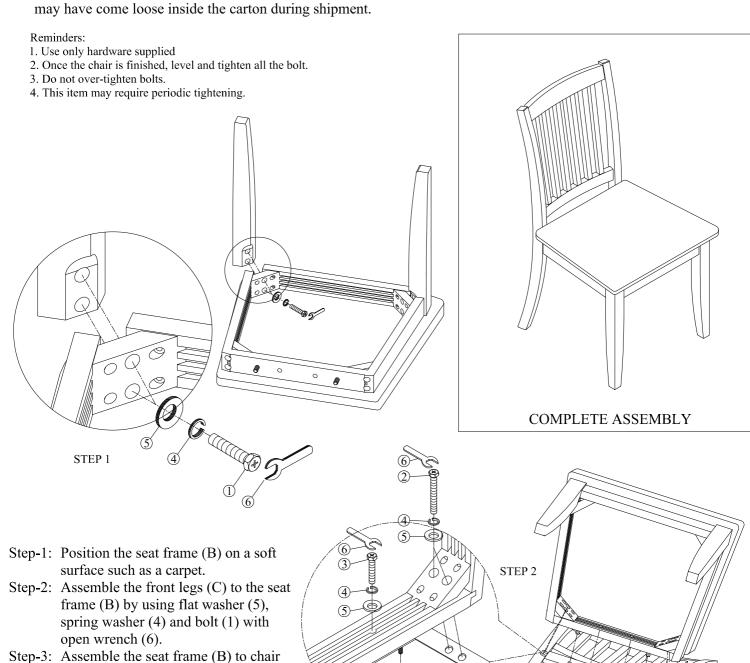
back (A) by using flat washer (5), spring washer (4) and bolt (2) with open wrench (6) for the corners and flat washer (5), spring washer (4) and bolt (3) for the back.
