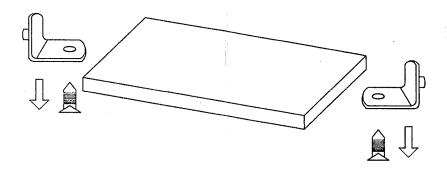
Please remove the screws from both clips in order to adjust the shelf to desired position.
