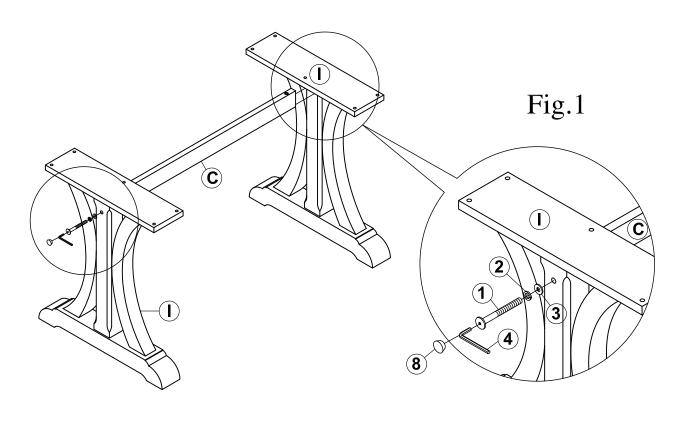
STEP 2: Attached Table Leg (I) to the Trestle Bar (C) using the provided hardware as shown on Fig.2.
