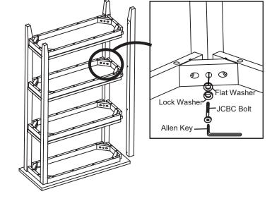
**STEP 2**Check its balance and tighten all bolts to complete the assembly.
