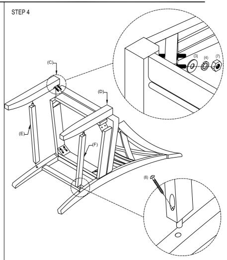
This step requires installation of four nuts and four screws
