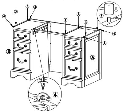
(5) Insert short (3/4") flat head wood screws (8 PCS) through metal figure 8 to connect Desk top (2) and pedestals.
