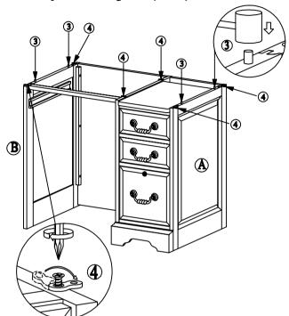
(5) Insert short (3/4") flat head wood screws (6 PCS) through Metal figure 8 to connect Desk top (B) and Desk base.
