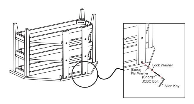
**STEP 4**Check its balance and tighten all bolts to complete the assembly.
