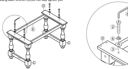
Step (3): Attach bottom rail (F) to the table leg (C), insert dowel wood (9), small washers (4), spring washers (6), short bolts (2), tighten by using allen wrench (8), do not fully tighten yet and put cap (G) into the hole of the table leg (C) as shown.
