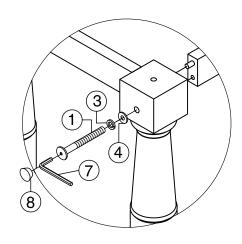
STEP 2: Attach Mounting Plate (E) to the Table Leg (C), insert short bolts (5), spring washers (3), flat washers (2) and tighten by using allen key (7).
