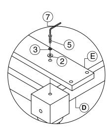
STEP 3: Attach Bottom Rail (F) to the Table Leg (C), insert short bolts (5), spring washers (3), flat washers (2) tighten by using allen key (7).
