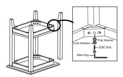
**STEP 2**Check its balance and tighten all bolts to complete the assembly.
